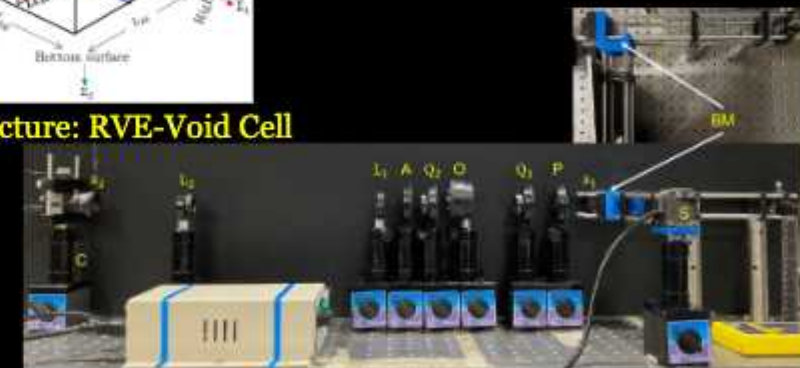
Ocular Mechanics: Invitro Digital Photo Elasticity Setup
