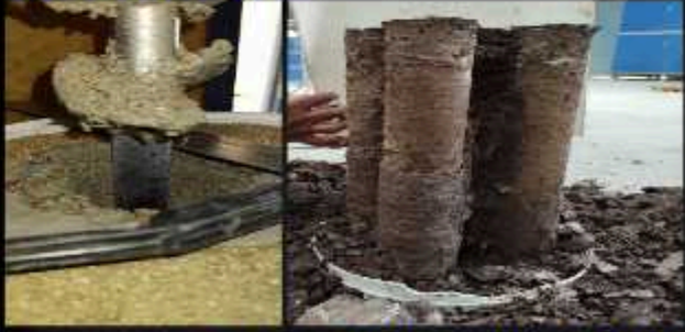
Scale-model DSM columns prepared in the lab
